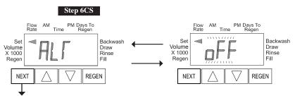
Step 6CS – This display will not appear if  $1.0\Gamma$  was selected in Step 2CS. Allows selection of one of the following using  $\blacktriangle$  or  $\blacktriangledown$ :
