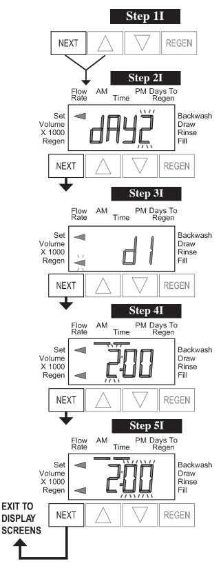
**Step 1I** - To enter Installer Display press NEXT and ▲ simultaneously for 5 seconds and release.
