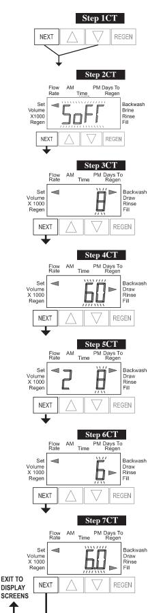
**Step 1CT** - Press NEXT and  $\nabla$  simultaneously for 5 seconds and release. If screen in Step 2CT does not appear, the lock on the valve is activated. To unlock press  $\nabla$ , NEXT, REGEN,  $\triangle$  in sequence, then press NEXT and  $\nabla$  simultaneously for 5 seconds and release.
